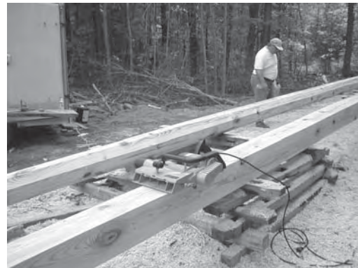
ASF made two 55' masts for Sidney Dickson's new bug-eye, the Katherine May Edwards
